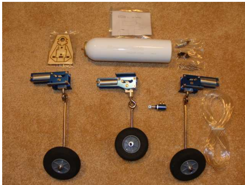
Fig. 17 - Spring Air retract kit that ships with the plane (July 2008)
